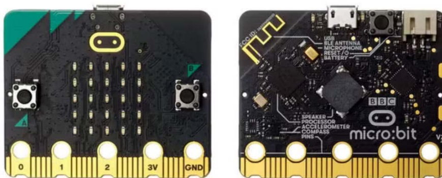
Figure 12. micro:bit V2 board (source: microbit.org [14])
