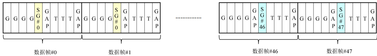
Figure 3. Schematic diagram of the NearLink ultra-short frame structure
