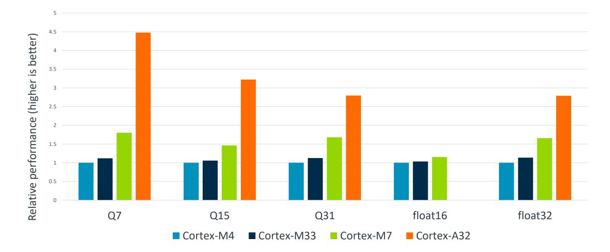
Simulation results using fast model and prototype compiler using selected CMSIS-DSP kernels such as CFFT, FIR, RFFT, matrix mul, vector dot product. Compared to Cortex-M4.
